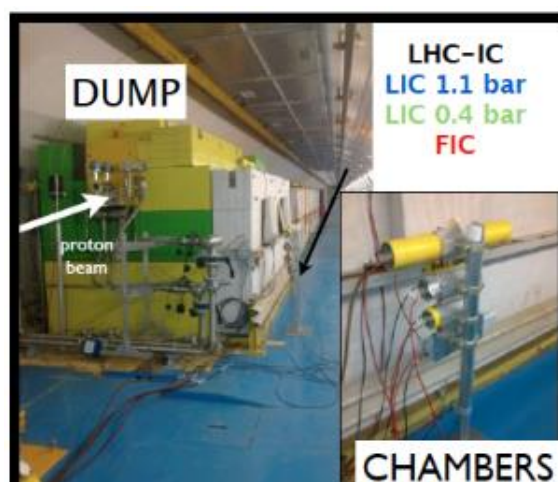
Figure 33: Example of BLM set-up in the experimental area. BLMs are positioned on and near the Beam Dump.
