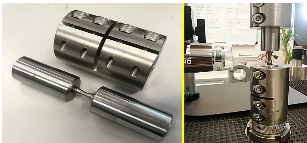
Figure 66: Dedicated holders for tensile tests showing dog-bone material specimens. POLITO
