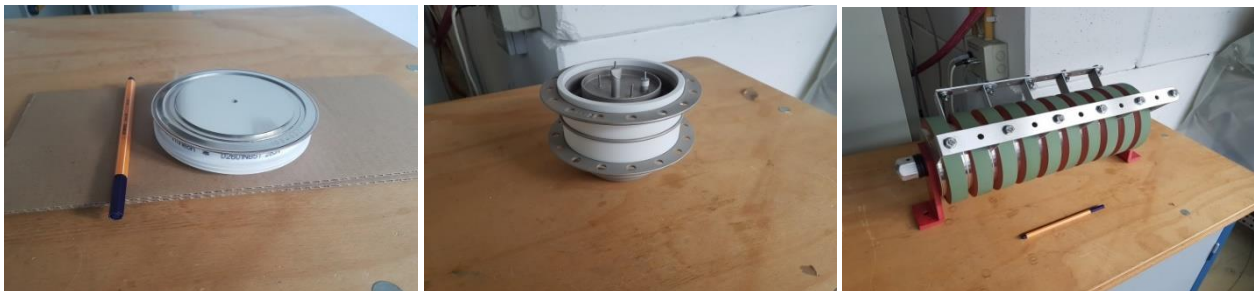
Figure 17: Pulse Diode, Pseudospark-Switch and Resistor (left to right)
