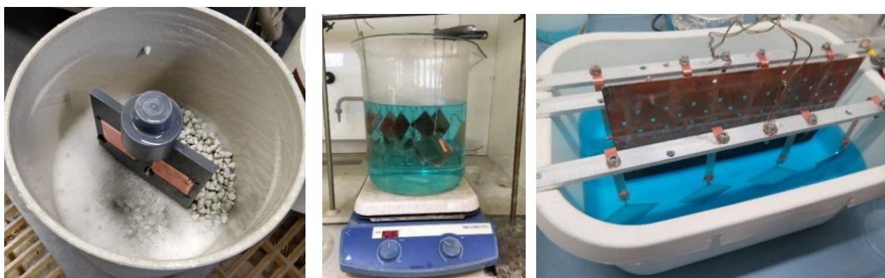
Figure 47: An overview of the polishing treatments configuration used: A) Tumbling, B) SUBU, C) Electropolishing
