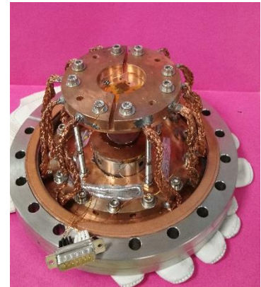
Figure 53: local AC-magnetometer at Saclay
