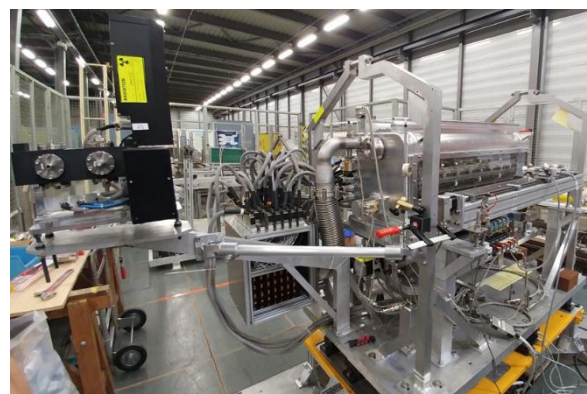
Figure 38: HRMT36 experimental tank with BTV/BPKG attached on the HRM table
