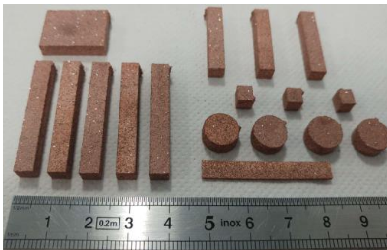
Figure 44: 17 samples of Copper-Diamond produced for thermophysical characterization at CERN
