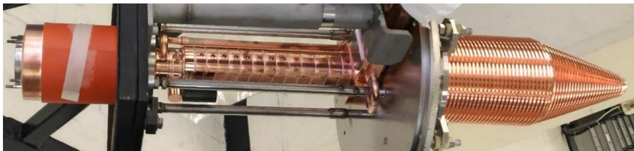
Figure 14: Manufactured kladistron prototype at 5 GHz
