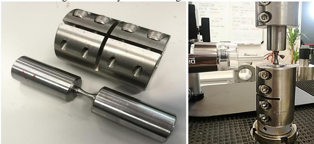
Figure 42: Dedicated holders for tensile tests showing dog-bone material specimens. POLITO
