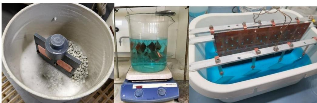
Figure 28: An overview of the polishing treatments configuration used: A) Tumbling, B) SUBU, C) Electropolishing
