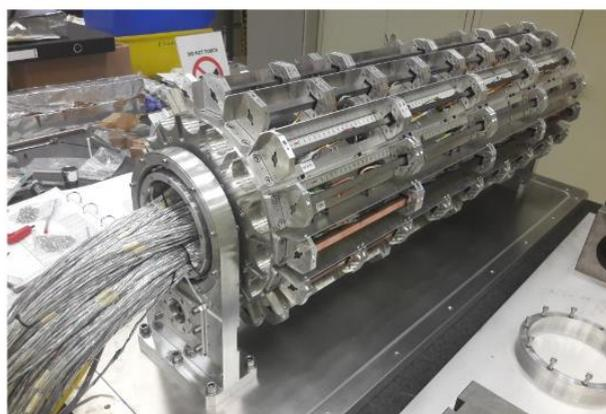
Figure 23: Illustration of the MultiMat experimental tank where the multiple target stations are shown on a rotatable barrel.
