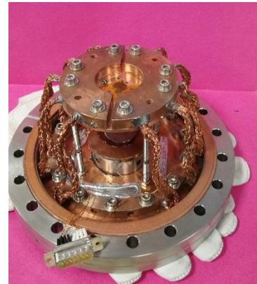
Figure 33: local AC-magnetometer at Saclay
