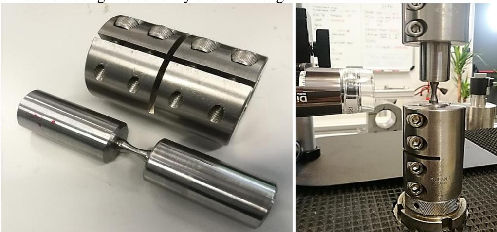
Figure 42: Dedicated holders for tensile tests showing dog-bone material specimens. POLITO
