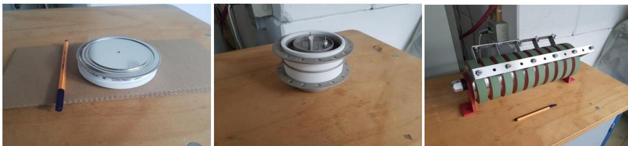
*Figure 10: Pulse Diode, Pseudospark-Switch and Resistor (left to right)*
