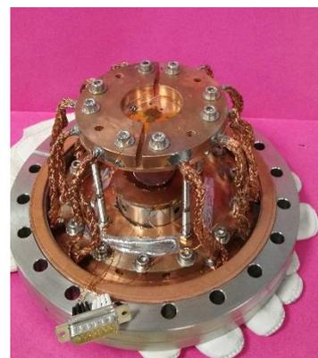
Figure 33: local AC-magnetometer at Saclay
